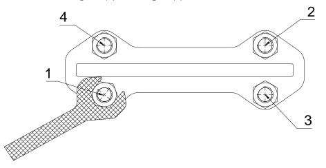
Figure 4: Tighten gland nuts crosswise
